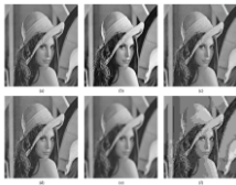
Fig. 8 Evaluation of "Low" images differently different scenes: (a) Original "Low" image: 112 × 112, (b) Contrast stretch image: 100 × 112, \alpha = 0.0772 , (c) Gaussian noise-contaminated image: 100 × 112, \alpha = 0.309 , (d) Impulsive noise-contaminated image: 100 × 112, \alpha = 0.6494 , (e) Blurred image: 100 × 112, \alpha = 0.346 , (f) PSF3 compressed image: 100 × 112, \alpha = 0.1676 .
